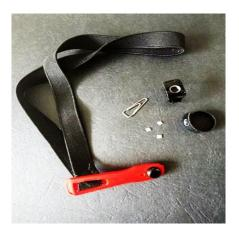
**Fig. 1**. The 'eye-D' holder used to measure eye lens dose (left) and the ring holder to measure extremity dose (right).
