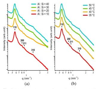
**Fig. 4.** SAXS scattering curves for sample series P (a) Al:Si ratio variation (b) Stirring temperature variation.
