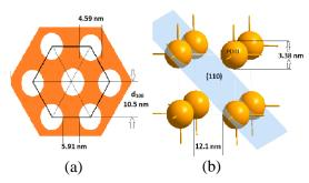
**Fig. 5**. Model of pore that formed on mesoporous silica material for (a) 2-D hexagonal structure and (b) cubic structure.
