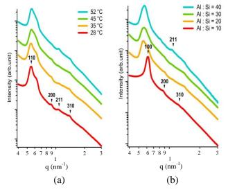
**Fig. 2.** SAXS scattering curves for sample series N (a) Stirring temperature variation (b) Al:Si ratio variation.
