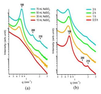
Fig. 1. SAXS scattering curves for sample series U (a)  $NaSiO_2$  variation (b) Sonication time variation.
