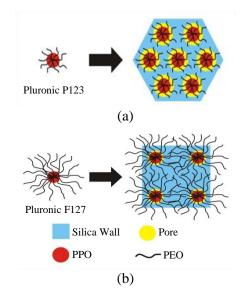
**Fig. 3.** Pore structure formation mechanism using two Pluronic types, (a) Pluronic P123 and (b) Pluronic F127.
