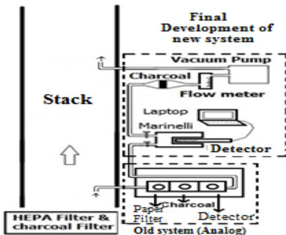
Fig. 2. Measurement system of  $^{131}\text{I}$  in the stack.
