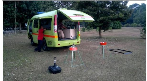
**Fig. 4.** Outdoor air measurement of  $^{131}\text{I}$  by direct method.
