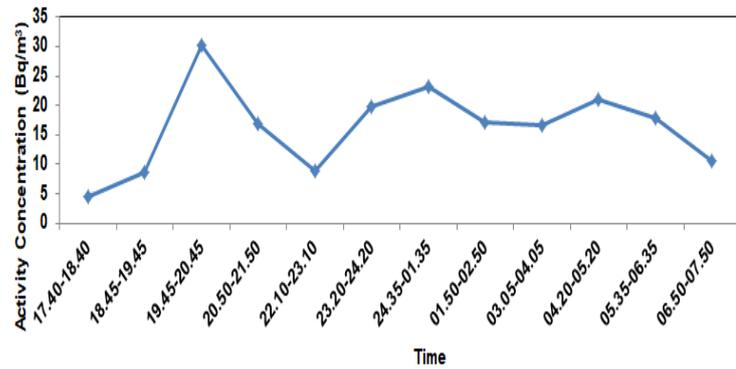
Fig. 9. <sup>131</sup>I activity concentration in the outdoor of the Puri Serpong housing complex by using indirect method.
