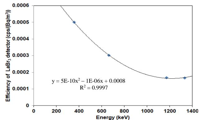
**Fig. 5.** LaBr<sub>3</sub> detector counting efficiency as a function of radiation source energy.
