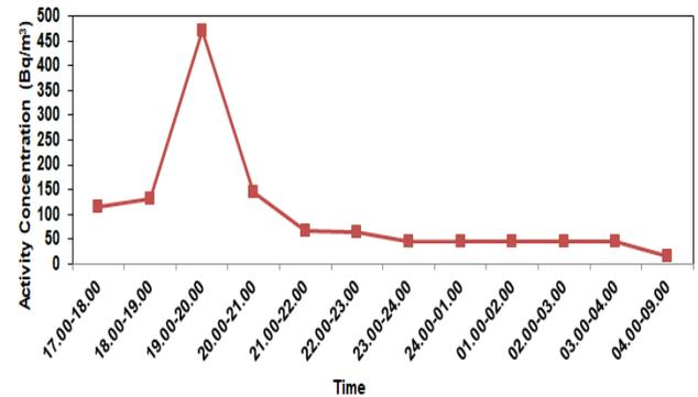
**Fig. 7.** Activity concentration of <sup>131</sup>I by using the indirect method on 11-12 December 2013 in the stack.
