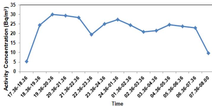
Fig. 10. <sup>131</sup>I activity concentration in the outdoor of the Puri Serpong housing complex by using direct method.
