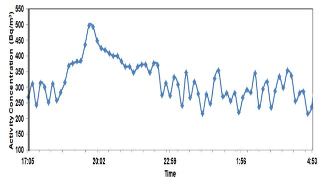
**Fig. 8.** Activity concentration of <sup>131</sup>I by using the direct method on 11-12 December 2013 in the stack.
