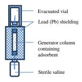
Fig.1. Radionuclide generator components.
