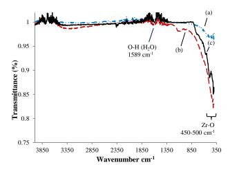
**Fig. 2.** FT-IR spectra of: (a) ZrOCl<sub>2</sub>•8H<sub>2</sub>O, (b) standard zirconia, (c) zirconia nanomaterial A.
