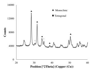
Fig. 4. XRD pattern of zirconia nanomaterial A.
