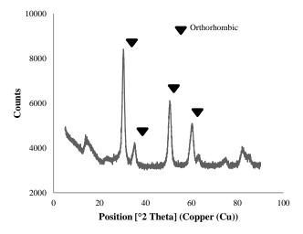
Fig. 7. XRD pattern of zirconia nanomaterial B.
