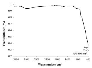
Fig. 5. FT-IR spectrum of zirconia nanomaterial B.
