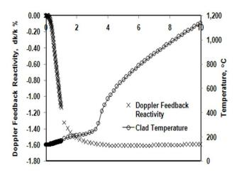
**Fig. 6.** Variation of cladding temperature with feedback reactivity for 1.85 % dk/k step reactivity.
