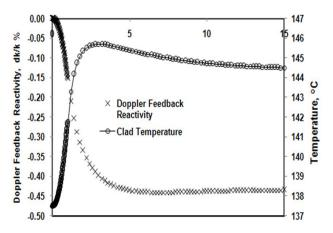
**Fig. 4.** Variation of cladding temperature with Doppler feedback reactivity for 0.5 % dk/k step reactivity.
