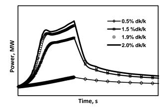
Fig. 1. Power transient behavior for different step reactivities.
