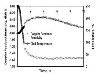
**Fig. 5.** Variation of cladding temperature with Doppler feed feedback reactivity for step 1.8 % dk/k.
