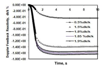
Fig. 3. Doppler feedback reactivity variation for different step reactivities.
