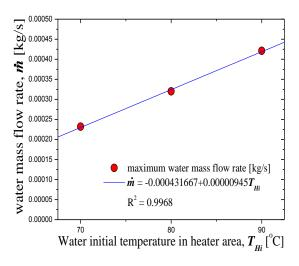
Fig. 10. High water mass flow rate base on initial temperature.
