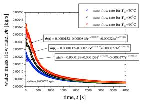
Fig. 7. Water mass flow rate characteristic.
