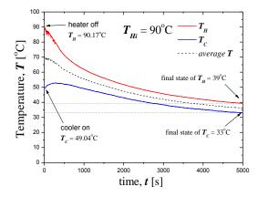
Fig. 5. Temperature measurement in heater and cooler area for initial temperature  $90^{\circ}$ C.
