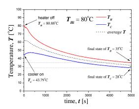
Fig. 4. Temperature measurement in heater and cooler area for initial temperature  $80^{\circ}$ C.
