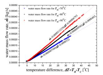
Fig. 9. Water mass flow rate versus temperature difference.
