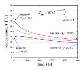
Fig. 3. Temperature measurement in heater and cooler area for initial temperature  $70^{\circ}$ C.
