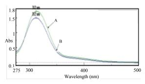
Fig. 2. Spectra of standard  $HAuCl_4$  in  $HCl\ 0.01\ M\ (A)$  and  $HAuCl_4$  from  $Au\ foil\ (B)$ .
