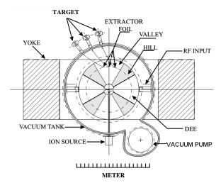
Fig. 2. The conceptual design of the 13 MeV Cyclotron: crosssection of the top view.
