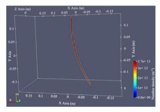
Fig. 6. Beam trajectory for scanning horn. The color indicates the number density of particles, with red means the densest region.
