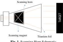
Fig. 1. Scanning Horn Schematic.
