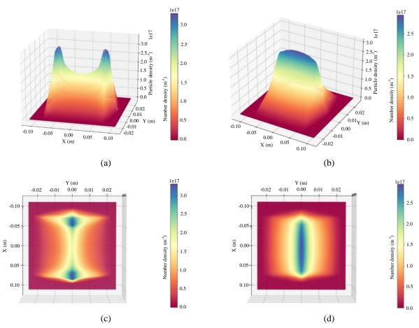
The irradiation distributions for triangular and sinusoidal signals are given in Fig. 7.
