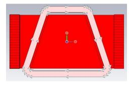
Fig. 2. Cross-sectional image of the scanning horn magnet.
