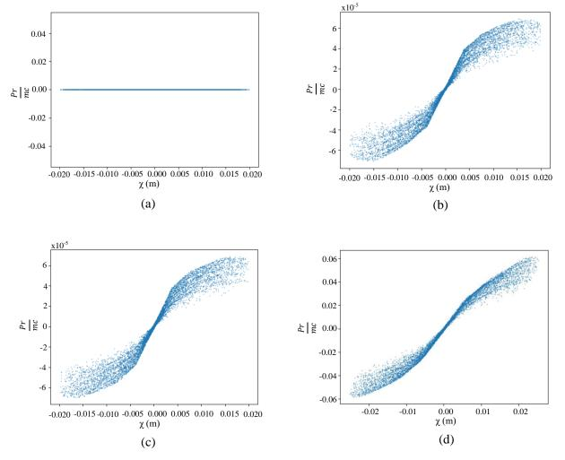
Fig. 5. Normalized emittance for (a) beam without particle-to-particle interactions; (b) 50 mA beam current; (c) 1 A beam current; (d) 50 A beam current.
