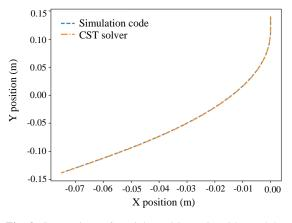
Fig. 3. Comparison of particle position using CST and the scanning horn simulation code.
