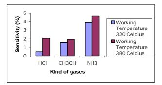
Fig. 4. Sensitivities of  $SnO_2$  thin film deposited using dc sputtering method at the conditions; operating pressure  $5x10^{-2}$  torr, anode-cathode voltage 2.0 kV, substrate temperature  $200^{\circ}C$  and deposition time one hour for various gas tested HCl, CH<sub>3</sub>OH, dan NH<sub>3</sub> working temperature  $320^{\circ}C$  and  $380^{\circ}C$ .
