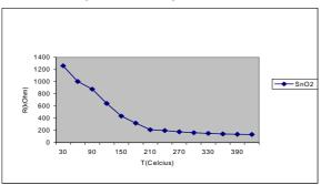
Fig. 1. Effect of temperature on the resistance of SnO<sub>2</sub> thin film.
