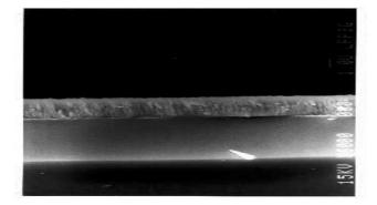
Fig.12. Cross section microstructure of  $SnO_2$  thin film deposited using *dc* sputtering technique for 1 hour and substrate temperature 200<sup>o</sup>C, magnification 600 x.
