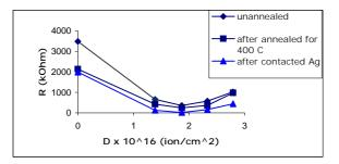
Fig. 3. Effect of annealing temperature on  $SnO_2$  thin films implanted with platinum for various dose at energy 60 keV.
