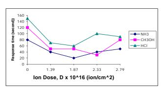
Fig. 7. Effect of platinum ion dose on the response time of  $SnO_2$  thin film at working temperature  $320^{\circ}C$ .
