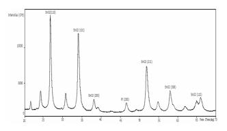
Fig. 9. XRD pattern of  $\text{SnO}_2$  thin film deposited using *dc* sputtering technique for 1 hour and substrate temperature 200<sup>o</sup>C and implanted by platinum ion at energy 60 keV, and ion dose  $1.87 \times 10^{16} \text{ ion/cm}^2$ .
