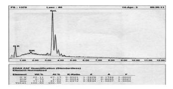
Fig. 14. Chemical composition of  $SnO_2$  thin film analyzed using EDX. The content of Sn and O element deposited on glass substrate are 31.62 at % and 67.17 at % respectively, while the rest (1.21 at %) is Si.
