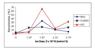
Fig.5. Sensitivities of SnO<sub>2</sub>:Pt thin film for various gas tested NH<sub>3</sub>, CH<sub>3</sub>OH, and HCl at working temperature  $320^{\circ}$ C and gas volume 0,769 (x10<sup>4</sup>) ppm.
