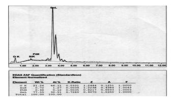
Fig. 15. Chemical composition of SnO<sub>2</sub>:Pt thin film analyzed using EDX. The content of Sn, O and Pt element deposited on glass substrate are 31.51 at % and 66.11 at %, and 0.12 at % respectively and the rest (1.27 at %) is Si.
