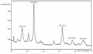
Fig. 8. XRD pattern of  $SnO_2$  thin film deposited using *dc* sputtering technique for 1 hour and temperature 200<sup>o</sup>C.
