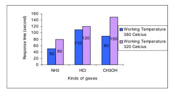
Fig. 6. The response time of  $SnO_2$  thin film to  $NH_3$ , HCl, and  $CH_3OH$  (methanol) for working temperature  $320^{\circ}C$  and  $380^{\circ}C$ .
