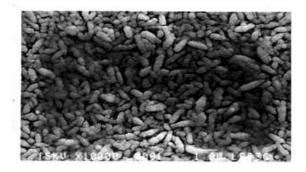
Fig.11. Microstructure of  $SnO_2$ :Pt thin film deposited using *dc* sputtering technique for 1 hour, substrate temperature 200<sup>o</sup>C and implanted by platinum ion at energy 60 keV, and ion dose 1.87 x 10<sup>16</sup> ion/cm<sup>2</sup>, magnification x 10,000.
