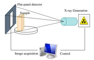
Fig. 1. Diagram of radiographic imaging system.
