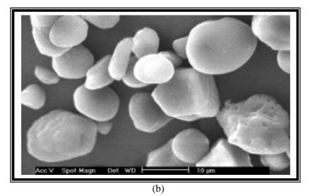
Figure 1. SEM of Sorghum Zh-30 starch: (a) Native sorghum starch; (b) Hydroxypropyl sorghum starch (MS 0.090).
