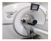
Fig 2. Placement of AAPM CT performance phantom during CT examination.
