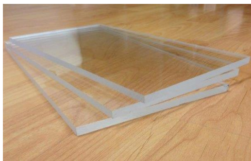
Fig. 3. Acrylic Phantom Material is clear plastic with the chemical formula (C_5H_8O_2)_n , polymethylmethacrylate (PMMA).
