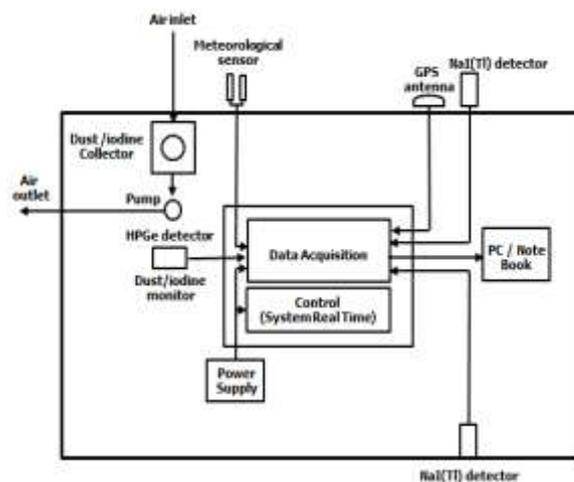
Fig. 1. Schematic diagram of the Carborne Survey Equipment.
