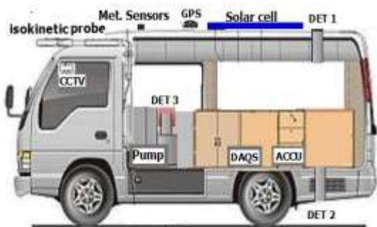
Fig. 2. Construction of a carborne survey equipment.
